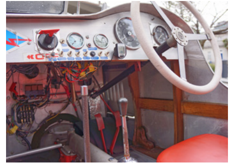
FAIR-WEATHER FRIEND MG TAs were made with a solid ash frame at Oxfordshire, like this 1937 model.
