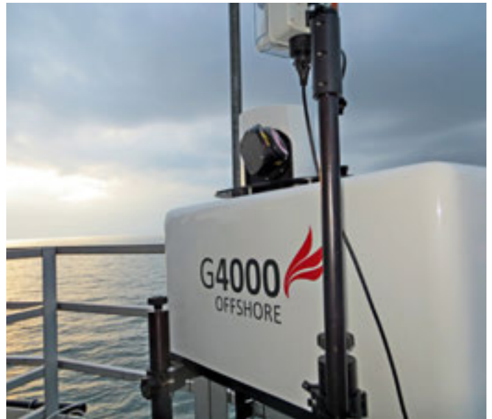
SgurrEnergy's devices measure turbine wind speed and direction.
